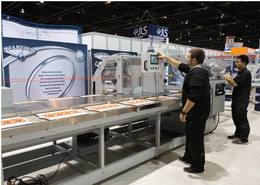
At Starview Packaging Machinery (Booth N-5325) , Steve Carlomusto, on computer, and Pei Jie Li ready the BSC 16-1418 carousel blister packaging machine.
